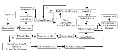
Fig. 3: Deep graph of the method safeClose() from Listing 2.
