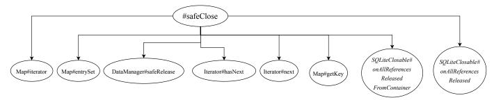
Fig. 2: Call Graph (CG) of the method safeClose() from Listing 2
