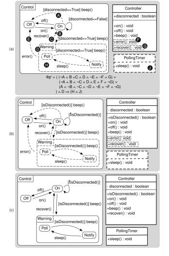
Figure 2: (a) The model P' after detail-adding refinement of P. (b) Refactored model P''  $(\Phi_{p''} = \Phi_{p'})$ . (c) Concretization M' of the partial model after uncertainty-removing refinement.
