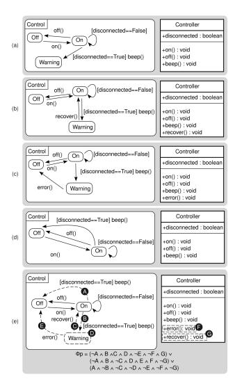
Figure 1: (a) An inconsistent model M. (b)-(d) Alternative repairs of M. (e) A partial model P capturing alternatives in (b)-(d). Dashed elements are optional.
