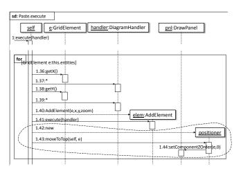
Figure 7. Our fix for the execute operation of the UMLet paste function.
