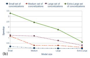
Figure 6. Speedup versus model size for different degrees of uncertainty: (a) experiment E1, (b) experiment E2.
